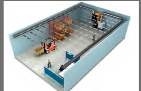
U-shaped Push-Pull System with 1 filter unit and 1 fan
